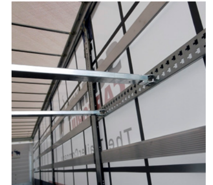
Load securing: wide range of options, such as the flexible load securing system.
