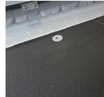
Non-slip floor simplifies load securing, meaning no non-slips mats and fewer lashings required.*
