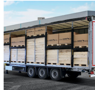
Double-decker: optimum use of space thanks to an easy-to-install second loading level for up to 67 pallets.*
