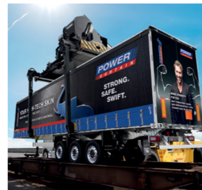
Combined transport: standardised gripper edges allow for vertical handling.*
