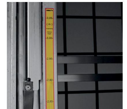
VARIOS body: height adjustment in 50 mm increments at the bulkhead from 2,700 to 3,050 mm and at the rear portal from 2,850 to 3,050 mm. Ideal for switching to different semi-trailer heights.*/**
