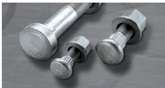
The high-strength knurled bolts from Schmitz Cargobull have longitudinal grooves on the shaft and thus wedge themselves into the bore. This also secures the connection against twisting.
