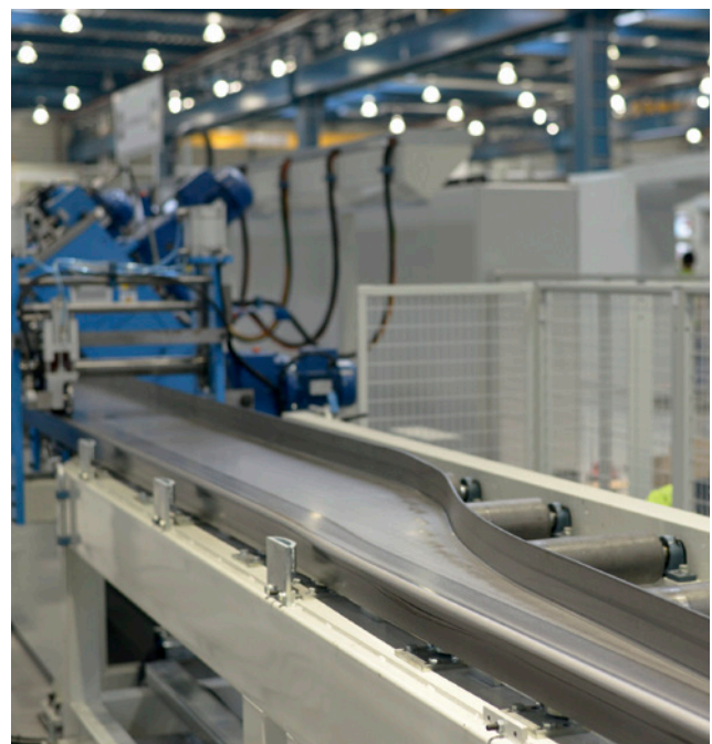
In the roller burnishing unit, the long beam is formed into its exact shape at room temperature by swivelling rollers.
