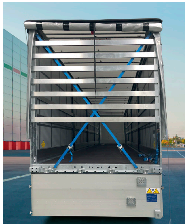
CODE XL rigidity due to diagonal tensioning cross and inserted aluminium slats.
