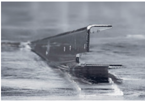
Only the finished workpiece is dipped into the zinc bath. This piece-galvanising process protects cut edges and cavities just as much as the large outer surfaces.
