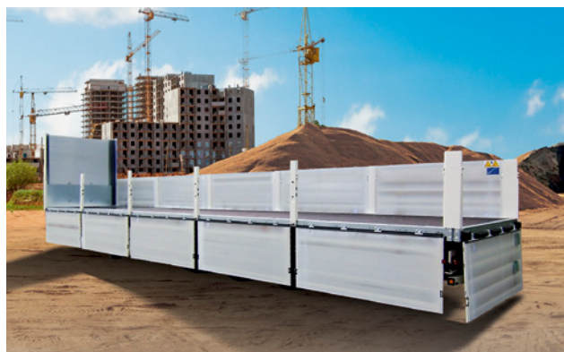
Fold-down drop sides and removable stanchions for full lateral loading through-loading width.
