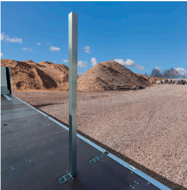
Hot-dip galvanised stanchion pocket magazines in the vehicle floor offer many possibilities for the arrangement of plug-in supports.
