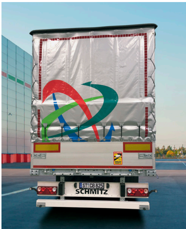
Prepared for transporting overlong freight: S.CS curtainsider semitrailer with dropside at the rear and roll-up tarpaulin.
