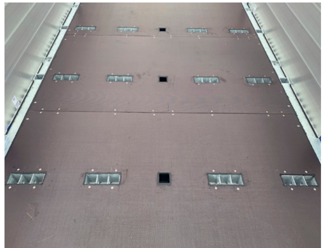
Even with the drop sides locked, the stanchion pockets in the outer frame remain completely usable.
