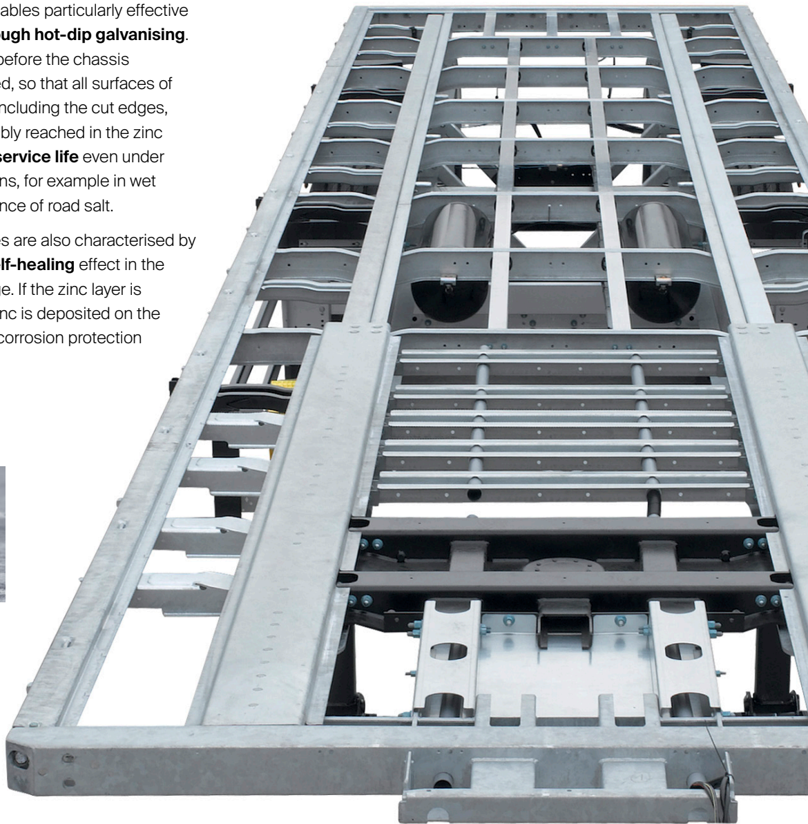
Only the finished workpiece is dipped into the zinc bath. This piece-galvanising process protects cut edges and cavities just as much as the large outer surfaces.
