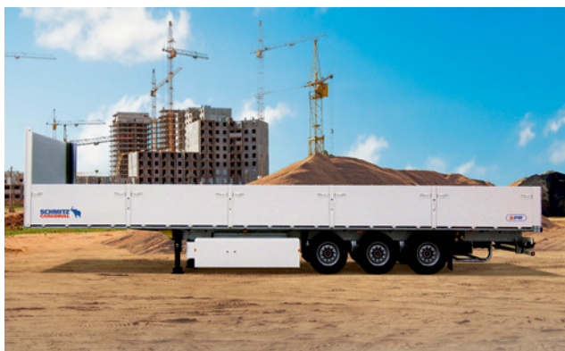
The S.PR BAU flatbed semitrailer with reinforced chassis and tight, easily removable drop sides.
