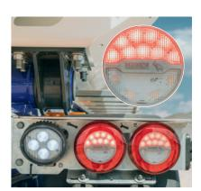
**LED three-chamber lights** in the Schmitz Cargobull design. As multi-chamber lights with dynamic turn signal. All rear lights in high lamp position as standard. LED worklights\*\* for illuminating the dumping area.
