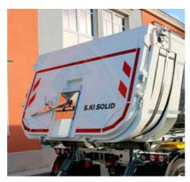
Overlying, thermally insulated pendulum flap is suitable for partial unloading. Optionally with asphalt pusher.
