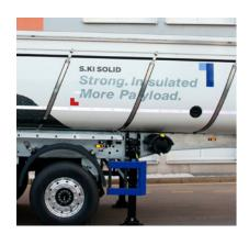
Cladding made of floating insulating sheets in case of external damage, individual segments can be quickly exchanged in the event of external damage.
