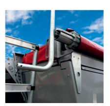
Roll-up tarpaulin with time-saving quickaction clamping device as simple and costeffective cover against wetness and drifts. Reduces air resistance.
