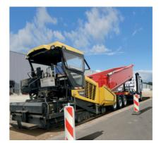
Optimized for tipping on the road paver: Foldable underride guard with high ground clearance for use on road paver. Optionally manually operated, or supported by spring mechanism for improved handling, or in electropneumatic version.
