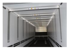
Extra-bright LED interior lighting in full body length on one or both sides for better visibility in the interior.
