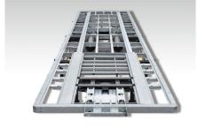
Rolled MODULOS chassis: Corrosion-resistant and easy to repair thanks to galvanisation and bolt technology.
