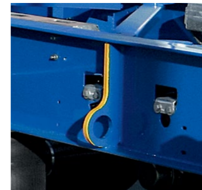
The semi-trailer container chassis can be equipped with ferry lashings* for use in ferry transport.
