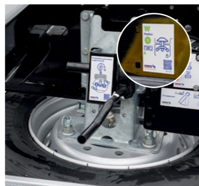
New labelling on locks and extensions for reliable identification of the different loading positions, supported by a loading plan and operating videos via QR code.
