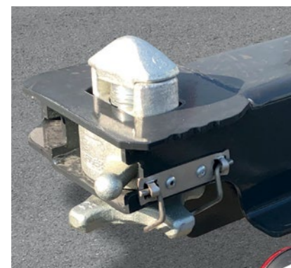
Standard TWIST LOCK locking mechanism: retractable and with anti-rotation lock
