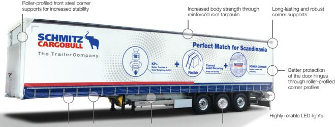
Trailer load at kingpin of up to 18 t Suitable for 3-axle tractor unit
