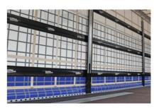
POWER CURTAIN\*: Body free from support laths for shorter loading and unloading times and greater operating safety.
