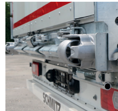
Ramp package Rear package protects rear portal and head frame from damage during loading. It consists of reinforcement of the head frame in the chassis as well as delta steel ramp bars and compressible roller ramp buffers.
