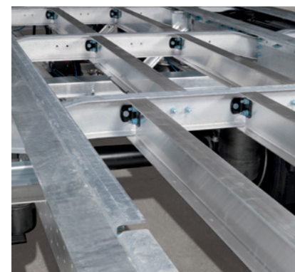
Rolled MODULOS chassis: corrosion resistant and repair-friendly design, thanks to bolted, hot galvanized technology.
