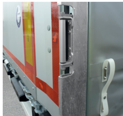
Integrated ram protection: riveted door hinges are better protected by the roller profiled corner supports at the rear
