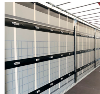
POWER CURTAIN: body without support laths for shorter loading and unloading times and greater work safety.
