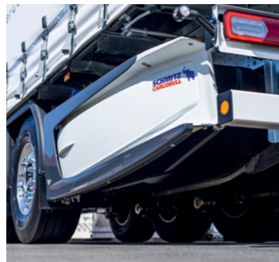
The lightweight and aerodynamically shaped storage box* ensures optimized airflow and contributes to further fuel savings. The large storage space offers room for pallets, spare wheels, etc.
