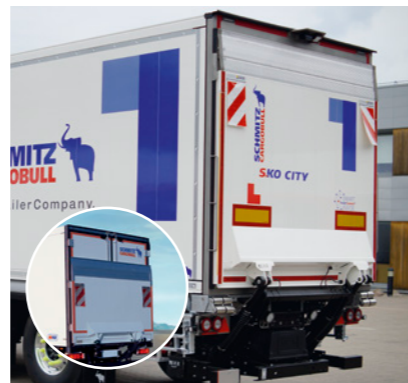
Tail lift* as rear closure. A two-wing tailgate with folded-forward or retractable tail lift* is standard.
