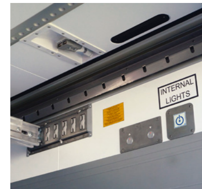
Interior control panel for light switches* and OptiLevel height adjustment* for ramp adjustment during loading and unloading.
