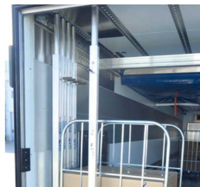
Magazines* for vertical and horizontal load-securing beams in the rear and under the ceiling simplify handling, fast load-securing and ensure safe transport.
