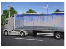
Efficient air distribution with three air ducts The interaction between the primary and secondary flow ensures a uniform temperature distribution for reliable cooled transport.
