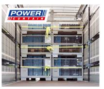
**Easy handling:** rear load securing using built-in tarpaulin loops in three rows e.g. for tensioning belts or safety tarpaulins.
