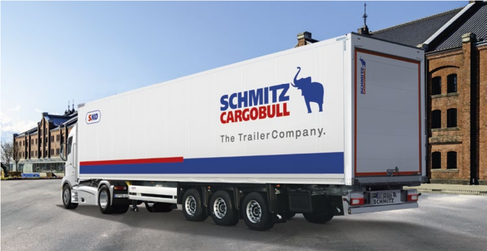
Spring-assisted or electric: a roller shutter lets you open the load compartment from the closed ramp.*
