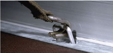
Additional load securing system in the cargo area: Lashing rings for tying down bulk goods.
