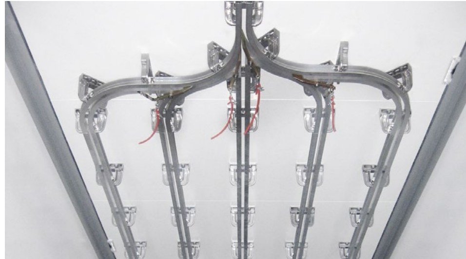
Special version on request: meat hanging system designed as a bi-rail system for use in the West European economic region. The roof and side walls of the FERROPLAST® box body are specially reinforced and can bear a weight of up to 24t across the whole of the roof area if the load is evenly spaced.
