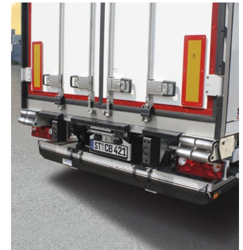
For loading and unloading at ground level: fold-under tail lift.*
