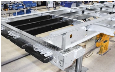
The additional longitudinal beams on the rear for greater stacker axle load.
