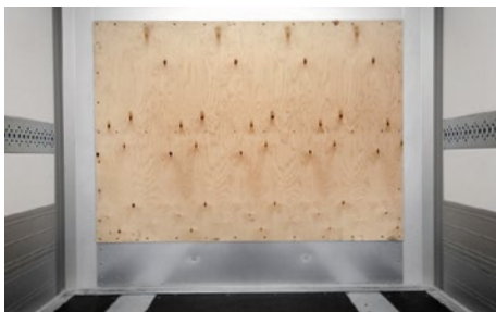
Reinforced bulkhead with a wooden plate and raised steel edge.
