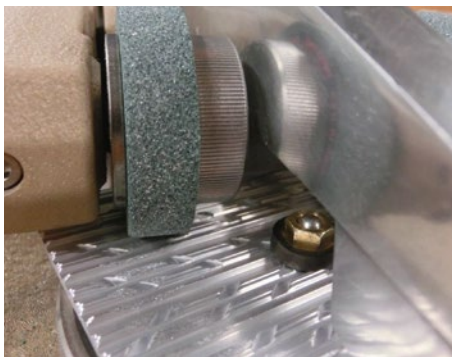
The Taber test uses a rotating, abrasive roller to test wear resistance.
