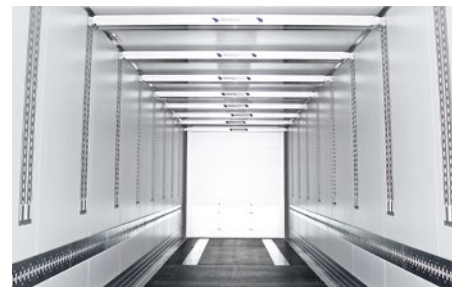
Double-decker system for 67 pallet spaces. Each support beam can bear up to 1,000 kg (see page 19).
