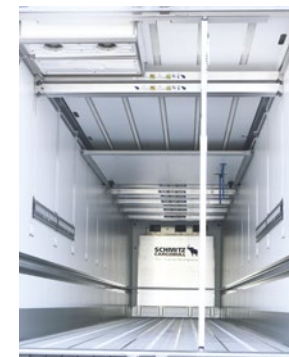
Vertical telescopic beams for load securing on the multifunctional floor.
