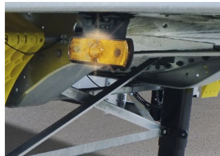
The side marking light with its flashing function is available as additional protection for cyclists and pedestrians.
