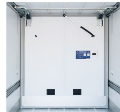
MultiTemp transports with swiveling partition* made of FERROPLAST®.
