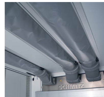
Robust air ducting system for uniform air circulation in the trailer, prevents the backflow of warm air and is easy to clean.
