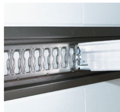
Load-securing rail allows free positioning of the load-securing beams along the entire length.
