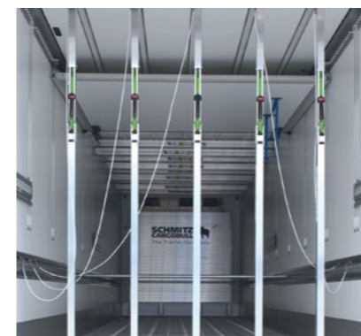
Vertical telescopic beams* simply and quickly in the multifunctional floor for load secured.
