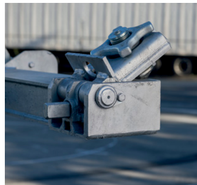
Folding latch as PIN latch for tunnel containers on the front beam.
