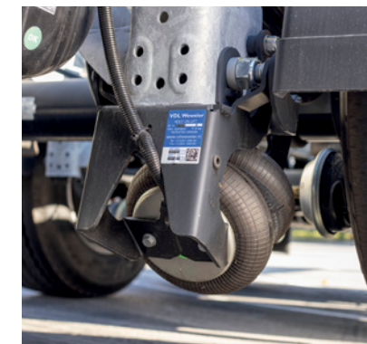
The lift axle* as a starting aid extends the wheelbase and thus increases the pressure on the drive axle. Unloaded in the lifted position, tire wear is reduced.
