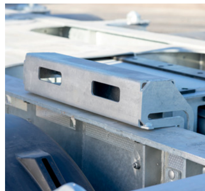
Three pairs of foldable container supports* for containers without tunnel
