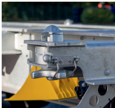
Twist Locks with protection against twisting on four pairs of container beams as standard locking.
