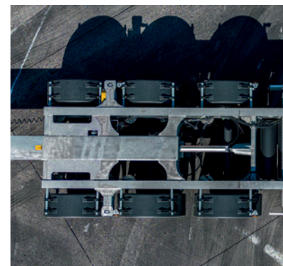
Long service life: Schmitz Cargobull container chassis are constructed from high-strength steel profiles and systematically protected against corrosion.
