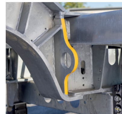
For use in ferry traffic, the semi-trailer chassis can be equipped with ferry lashings .
