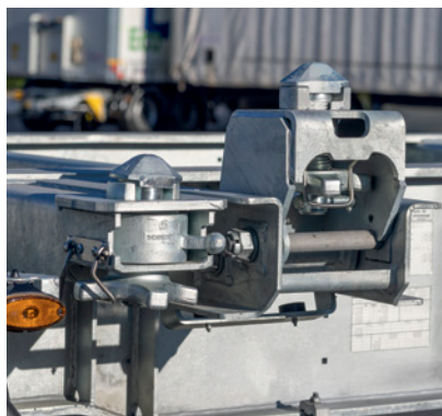
With 2 x 20' loads, two KLAPP LOCKS take over the rear locking of the front container.
