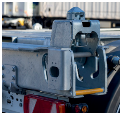
Two STEP LOCKS® on the rear extension adjust your semitrailer chassis in two easy steps.
