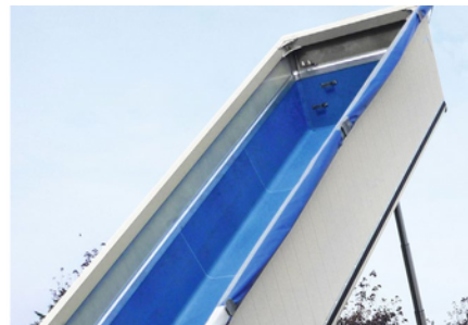
The plastic lining * protects against wear, offers good sliding properties and reduces the risk of freezing.
