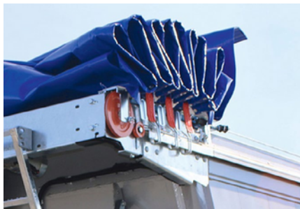
The sliding roof * enables time-saving opening and closing. Available in a manual or electric version, operated by remote control.
