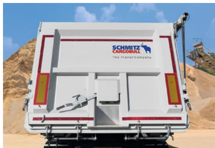
The surface-mounted swing flap is suitable for partial unloading and is optionally available with a slider. The combination door with swing and door function or swing flap with chute extend the range.
