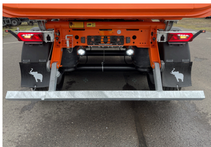
The folding underide guard with high ground clearance enables use on road pavers and can be operated manually, optionally available with a spring mechanism for easy handling or in a pneumatic version for increased safety and time savings.
