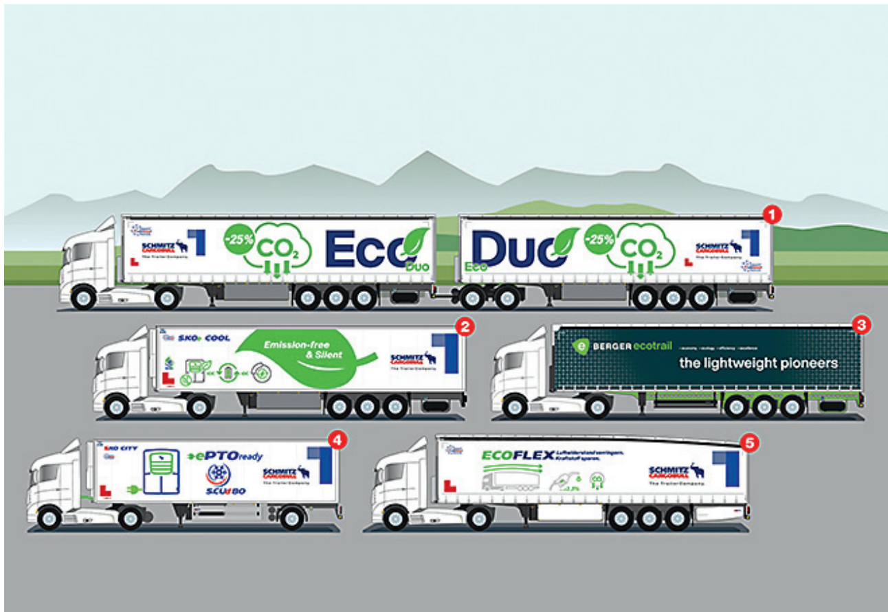
1. EcoDuo concept: one tractor unit with two standard trailers 2. Type-approved, all-electric S.KOe COOL refrigerated box body semi-trailer 3. BERGER ecotrail® lightweight semi-trailer 4. Diesel-powered cooling unit ePTOready: emission-free with eTruck 5. EcoGeneration: aerodynamic curtainsider semi-trailer and box bodies to reduce consumption and carbon emissions
