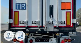
The TL4 door locking system in the S.KO COOL refrigerated box is PINsecured and can be locked and unlocked remotely using the TrailerConnect® portal. On site, the driver can enter the PIN using the beSmart app or on the display of the S.CU refrigeration unit. The automatic geo-lock uses the telematics geofencing monitoring to allow access only in defined zones.
