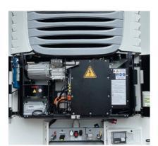
**Electric refrigeration unit S.CUe** with 15,800 watts cooling capacity, 10,500 watts heating capacity. The charging and battery management system ensures full practicality.
