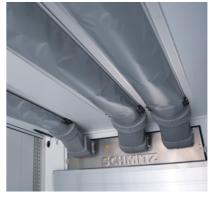
**Efficient air flow** - for uniform temperature control in the entire cargo hold - reduces energy consumption and ensures greater cargo safety.
