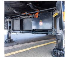
**Battery Power Pack** with a capacity of 32kW/h. The lithium iron phosphate battery transformer has a self-sufficient running time of approx. 4.5h and requires approx. 2h for a full charge.
