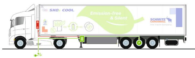
Charging options for the battery in the support winch of the S.KOe semitrailer box:
