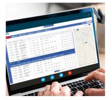
**TrailerConnect® telematics portal** allows refrigeration unit control with setpoints for operation, temperature and alarm management. It provides information about the battery's state of charge, the vehicle's position and is used for route planning.
