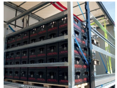
Load secured positively to the front with securing beams and supports, which are secured with diagonally tensioned belts .
