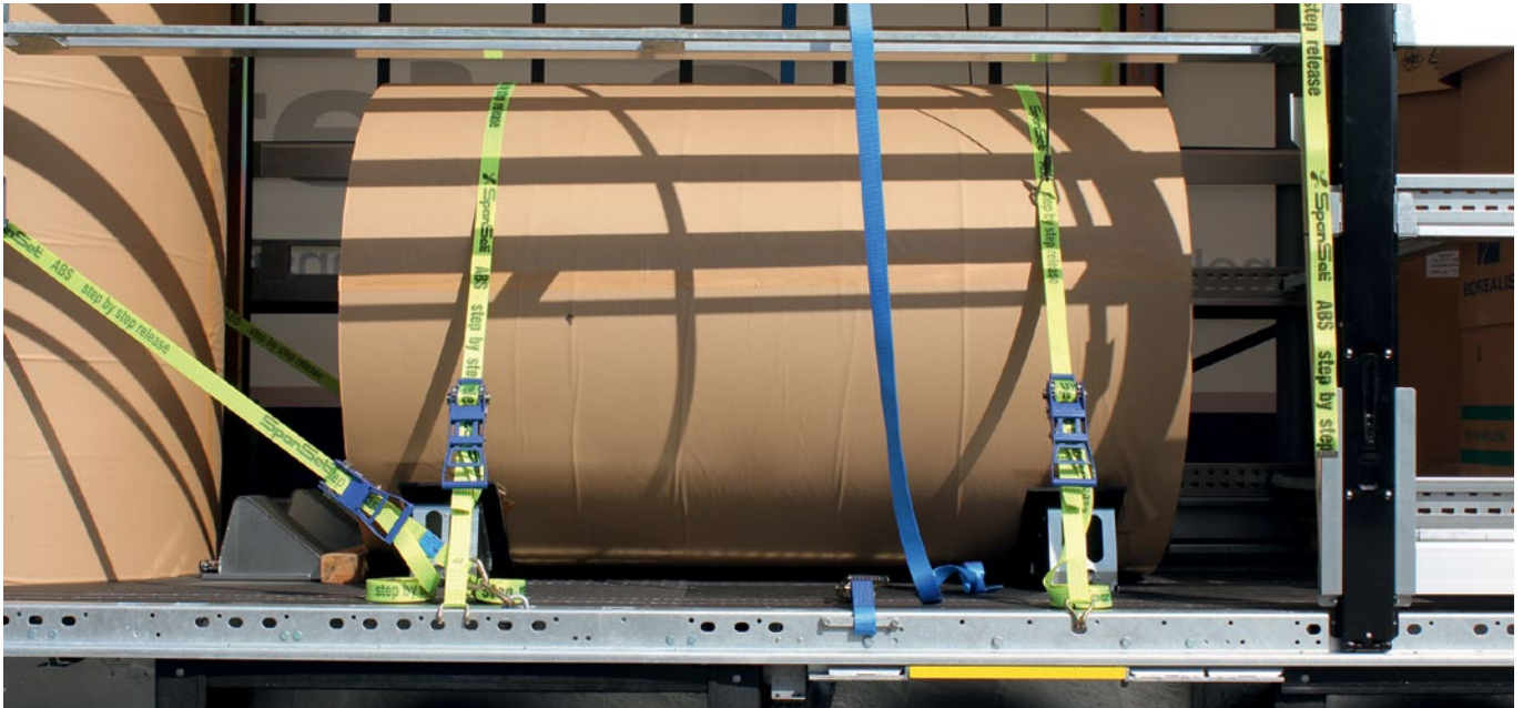
Horizontal paper roll lengthways to the direction of travel. Lashed down with 2 belts and secured at the front with securing wedges
