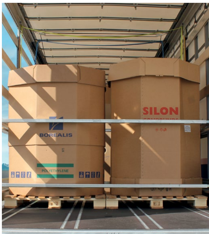
Octabin Some loads are not suitable for lashing down because the packaging would not withstand the pressure. In the case of octabins, for example, form-fit securing must be realised on all sides.
