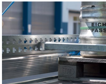
Horizontal load-securing beams limit the load for partial loads. The double slats inserted at the bottom provide a high, lateral stop for palletised freight.
