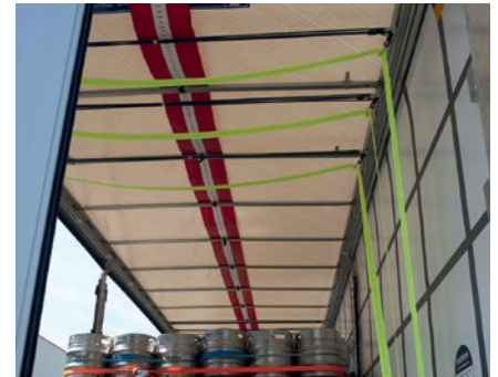
The sliding lashing system fitted between the roof bars enables customised load securing. Sliding retainers accommodate load securing straps. This means they can be moved to any position in the load compartment.
