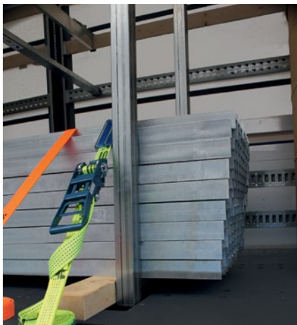
Examples of the use of vertical supports for load securing for pallets and general cargo.
