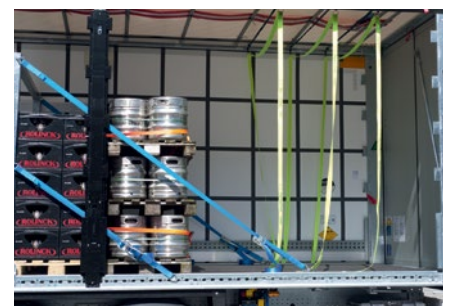
When not in use or loaded, the load securing straps are simply moved or pulled through the retainers under the roof, leaving the load compartment free. This means they can be moved to any position in the load compartment.
