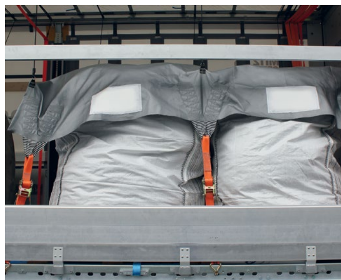
Form-fit securing for flexible big bags: lower side slat made of aluminium and tarpaulin with lashing straps.
