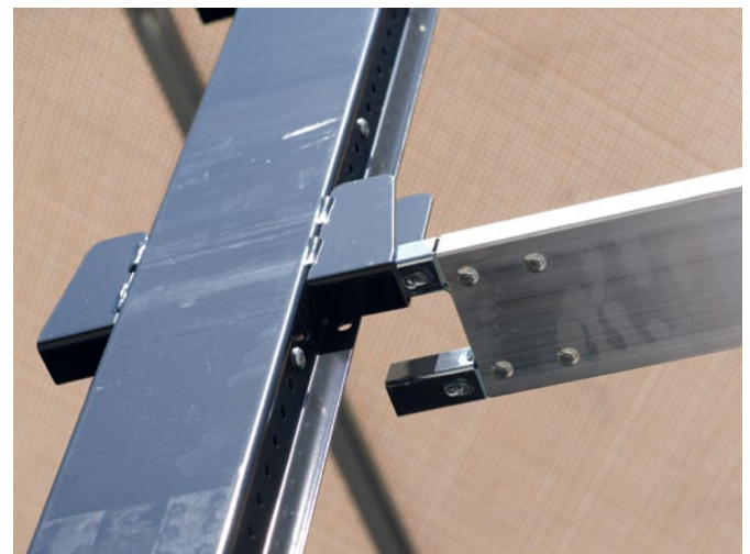
Both pictures above: Slat with hinged spacer for transporting well boxes.
