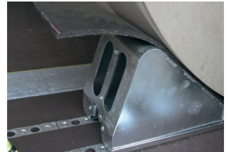
Positive locking of the castor using special wedges in conjunction with anti-slip mats.
