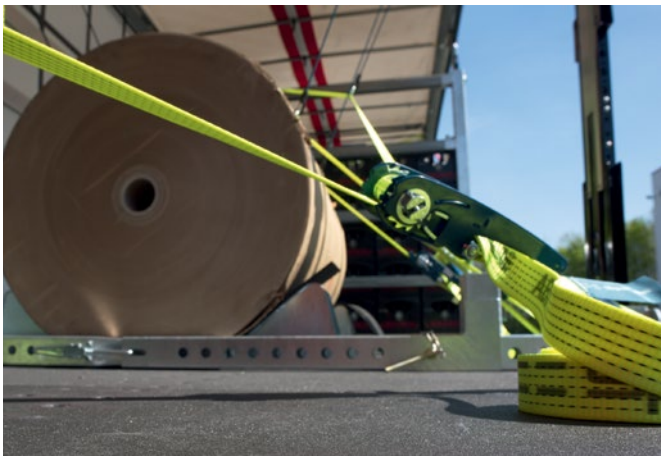
Additional securing of the paper roll to the front and rear.
