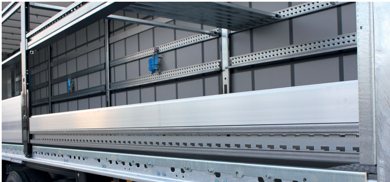
Steel slats with a close-meshed grid for attaching crossbars and belts allow any desired division. Aluminium slats can be used to form a stable side wall.
