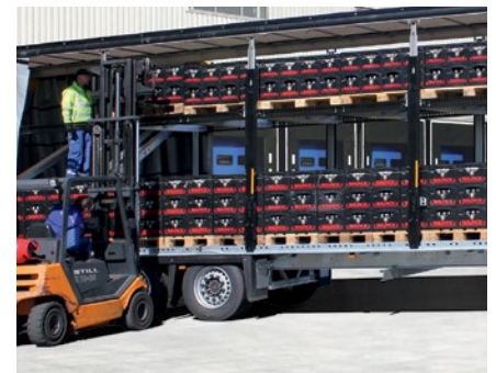
Two pallets can be stacked one on top of the other for banded drums. Two pallets with beverage crates require double-decker equipment on top of each other.
