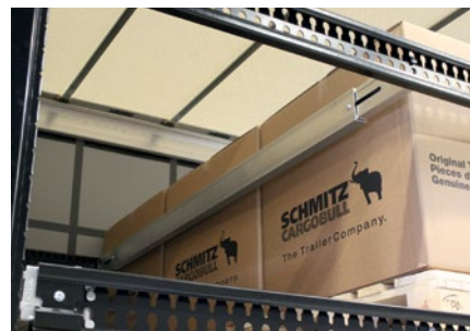
Load securing with crossbars
