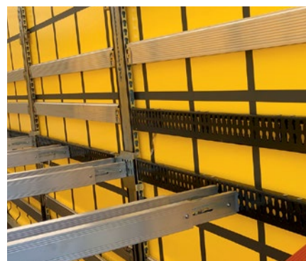
Load securing with crossbars
