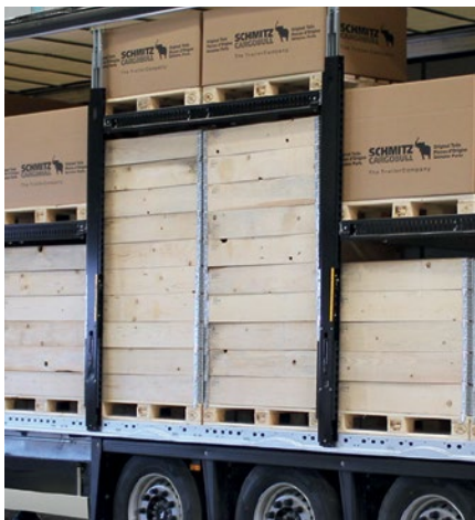
Example of a form-fit load with alternating levels . The double-decker height can be individually defined between the stanchions in some systems.
