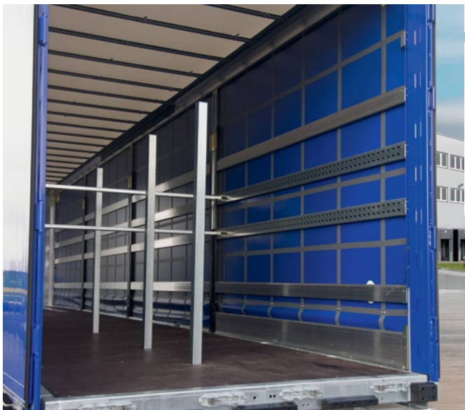
For transporting profiles and bar material: additional stanchions and steel support slats with horizontal beams.
