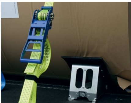
Wedges positively secure a paper roll, lashing straps increase the contact pressure.
