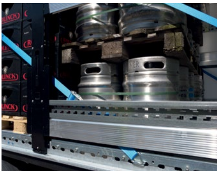
Barrelled goods, banded and unbanded, can be transported safely without lashing down if the appropriate equipment is used.
