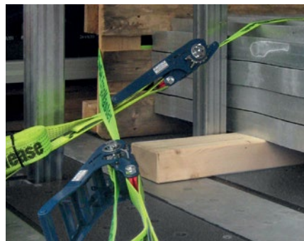
Form-fit secured to the side and to the front and lashed down.
