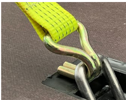
Flush with the floor, this allows lashing down of up to 4 tonnes from the surface
