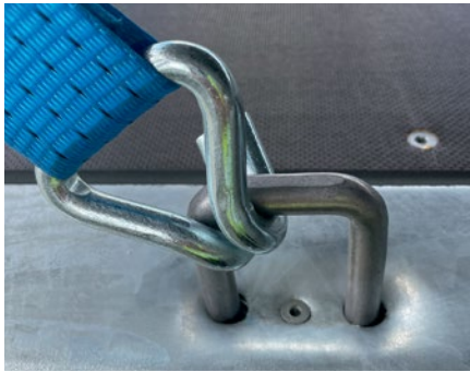
Various end fittings are possible on the straps. Here is a pointed hook that engages in a retractable lashing eye on the outer frame.
