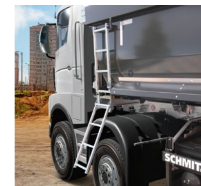
Extensive additional equipment to choose from: side ladder for load inspection.
