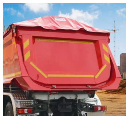
The recessed pendulum flap with chute for central unloading.
