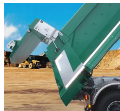
Ideal for coarse and abrasive bulk goods: the hydraulic tailgate.
