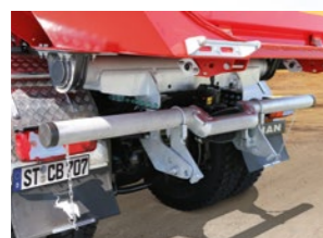
Optionally available: Offset, folding underride guard for vehicles with trailer coupling
