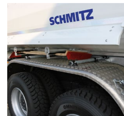
Side fender plates to protect personnel from falling materials during loading and unloading. Holder for the storage of brooms and shovels.
