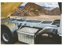
Safety, durability and costeffectiveness The tipper truck bodies can be optimally combined with the selected trucks. The galvanised, torsionresistant subframe allows the truck to be mounted on all common makes of truck, transforming the vehicle into a highly resilient, safe and efficient unit.
