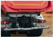
**Optionally available** Fold-down, hinged underride protection for vehicles with a towbar.
