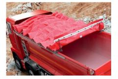
Electric sliding roof Easy and quick to operate from the cab. The convenient roll-top cover, operated from the ground, is also available.
