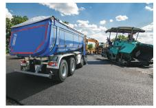
The proven **thermal insulation**, as used in tipper trailers, is also available for the M.KI in selected height and length combinations.
