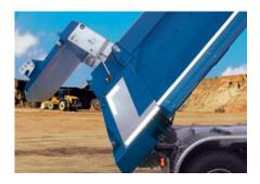
Hydraulic rear wall As a surface-mounted rear wall flap, it is ideal for coarse bulk materials.
