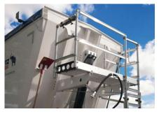
Safe and practical: the **height-adjustable** working platform with non-slip floor, access aid for the skip and parking position for the hydraulic hose
