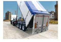
The **curved roller curtain** is easy to handle and can be closed from the ground using the long centre tensioning strap. Emptying with the curtain closed using the swing function of the combi door saves time. The arched shape with stabilising central tube also prevents water from collecting
