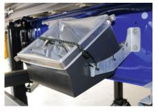
**Grain outlet hopper f**or grain pusher with practical parking position on the chassis or protected in the storage box.
