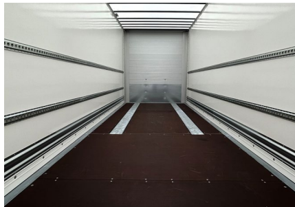
Robust screen-printed floor: The standard floor load capacity is 5.5t. The vehicle is also optionally available with a floor load capacity of 7.1t or 8.0t if heavier loads are being transported or industrial trucks are being carried.
