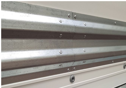
Robust heavy-duty base scuff plate to protect the sidewall and speed up the loading processes.
