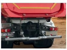
**Optionally available**Fold-down, hinged underride protection for vehicles with a towbar.
