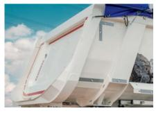
Interior swing flap with a chute. A surface-mounted swing flap with all-round seal is also available as a variant.
