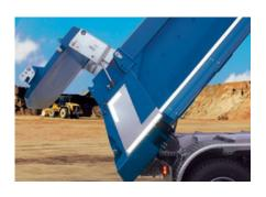
**Hydraulic rear wall**As a surface-mounted rear wall flap, it is ideal for coarse bulk materials.
