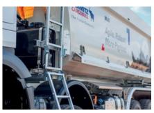
Extensive range of additional equipment options, including side access ladder for loading control and brush and shovel holder.
